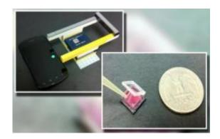
The ePetri platform is built from Lego blocks and uses a smartphone as a light source. The imaging chip is seen in detail on the right. Credit: Image courtesy of Guoan Zheng, California Institute of Technology
