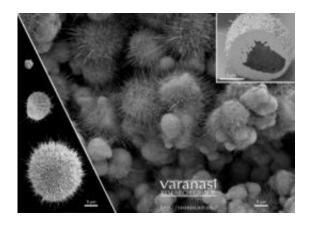
Images taken with a Field Emission Scanning Electron Microscope show the nanowire bristles that form on copper particles of different sizes. At top right, a cross-section of one of the particles reveals its hollow interior. Image courtesy of the Varanasi Lab
