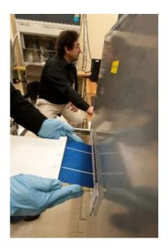
An NREL colleague inserts a multi-crystaline silicon solar cell sample into the Optical Cavity Furnace while Principal Engineer Bhushan Sopori, gets ready to read its analysis on his computer screen. Credit: Dennis Schroeder
