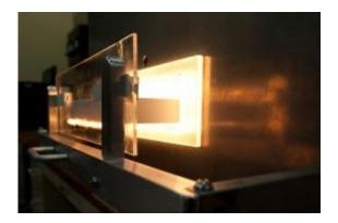
The cavity inside the Solar Optical Furnace glows white hot during a simulated firing of a solar cell. Credit: Dennis Schroeder
