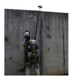
The Recon Scout XT robot can be attached to the SearchStick to survey environments while keeping soldiers in relatively safer positions. Image credit: ReconRobotics
