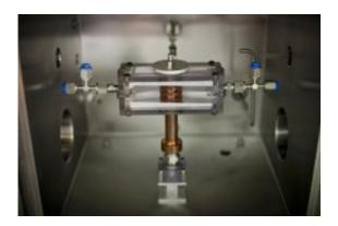
This laboratory setup was used to test the principles behind Wang and Miljkovic's concept for a hybrid solar thermoelectric system that could deliver both electricity and heat. Photo: Dominick Reuter
