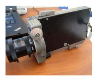
This Data Acquisition Camera (DAC) was one of two 16mm cameras on the Apollo 14 lunar module "Antares" when it landed on the moon on Feb, 5, 1971. Credit: FLSD
