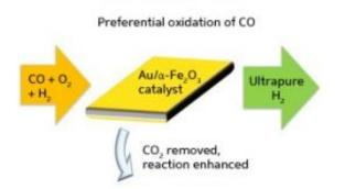
A combined catalyst/carbon dioxide (CO2)-sorbent system (middle) that removes carbon monoxide (CO) contaminants from hydrogen gas (H2) may soon be part of on-board fuel cells. Credit: A\*STAR
