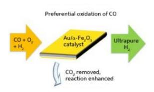
A combined catalyst/carbon dioxide (CO2)-sorbent system (middle) that removes carbon monoxide (CO) contaminants from hydrogen gas (H2) may soon be part of on-board fuel cells. Credit: A\*STAR
