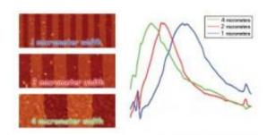
At a constant carrier density, varying the width of the graphene ribbons -- from 1 micrometer (millionth of a meter) to 4 micrometers -- changes the plasmon resonant frequency from 6 to 3 terahertz. The spectra of light transmitted through the device (right) show corresponding absorption peaks. Credit: Lawrence Berkeley National Laboratory
