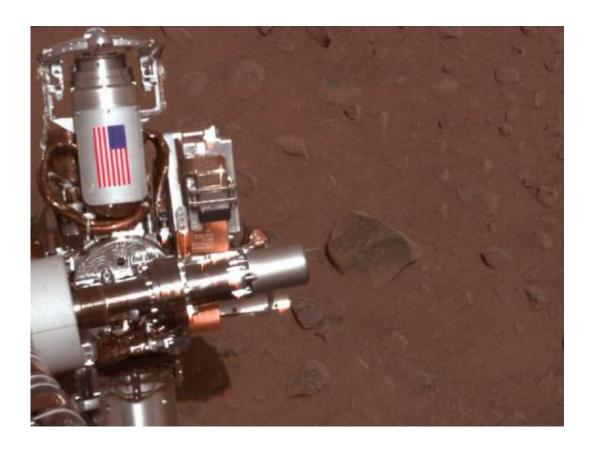
The piece of metal with the American flag on it in this image of a NASA rover on Mars is made of aluminum recovered from the site of the World Trade Center towers in the weeks after their destruction. Credit: NASA/JPL-Caltech/Cornell University
