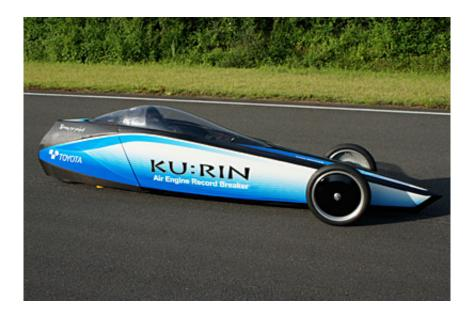
(PhysOrg.com) -- Toyota Industries intends to apply for a Guiness World record for the fastest car driven by a compressed-air engine, after its Ku:Rin, as the vehicle is called, reached 129.2km/h (80.3 mph)on a test run earlier this month. This is a three-wheel, one-seater vehicle that broke the speed record for compressed air-powered vehicles at the Japan Automobile Research Institute test facility.
