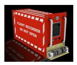
An airplane's digital flight-data recorder, or "black box," holds massive amounts of data, documenting the performance of engines, cockpit controls, hydraulic equipment and GPS systems, typically at regular one-second intervals throughout a flight. Inspectors use such data to reconstruct the final moments of an accident, looking for telltale defects that may explain a crash.
