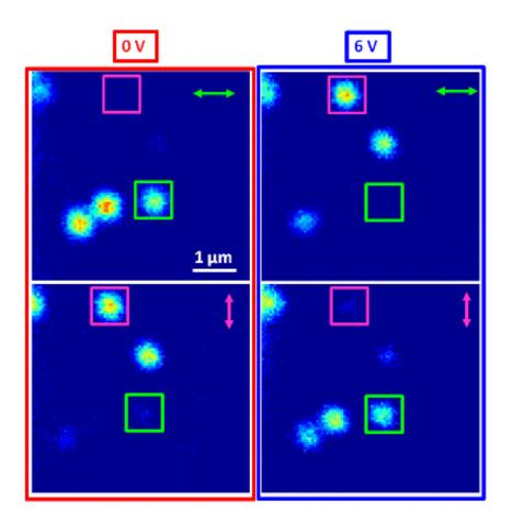
Polarized dark field scattering images of single gold nanorods in electrode gaps show them either turned on or off depending on voltage applied to a swarm of liquid crystals. The arrows indicate the polarization of detected light, either parallel (purple) or perpendicular (green) to the electrode array. (Credit Link Lab/Rice University)
