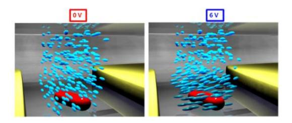
Applied voltage creates a nematic twist in liquid crystals (blue) around a nanorod (red) between two electrodes in an experiment at Rice University. This graphic shows liquid crystals in their homogenous phase (left) and twisted nematic phase (right). Depending on the orientation of the nanorods, the liquid crystals will either reveal or mask light when voltage is applied. (Credit Link Lab/Rice University)
