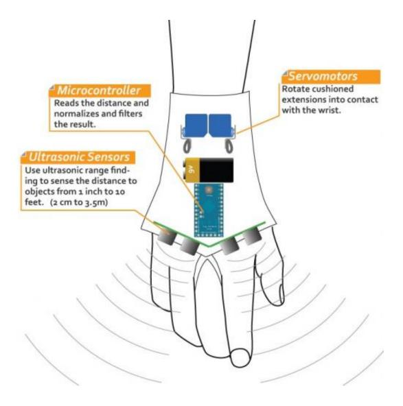
As for device accuracy, Hoefer says that lasers would have provided the most accuracy, but would be too costly, in his opinion. The cost of materials for Hoefer's prototype is \$65. "For now ultrasonics work best at this price."
