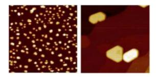
Physicists at the U.S. Department of Energy's Ames Laboratory have discovered that rare-earth materials, such as dysprosium (shown at left), and other materials, such as lead (shown at right) behave differently when a few atoms of each type of material are deposited on a graphene and the atoms self assemble into tiny islands. Rare earths appear to move slowly, suggesting strong electronic interaction, while lead moves quickly, suggesting weaker electronic interaction.
