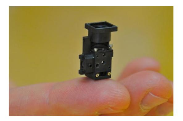
Researcher Mark Schnitzer demonstrates the microscope's tiny size and weight.
