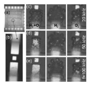
Formation of bubbles at the electrodes during electrolysis (can be seen in a and b). Situations c, d, and e show the formation of both hydrogen and oxygen on the left, hydrogen alone in the middle and oxygen alone on the right. Situation e shows combustion taking place on the left. No bubbles can be seen on the electrodes.
