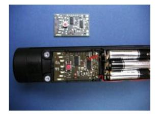
Heinrich Iglseder adapted his space sensor for a regular vacuum cleaner. The sensor is mounted in the extension tube and its electronics are mounted in the vacuum cleaner handle. Credits: H. Iglseder
