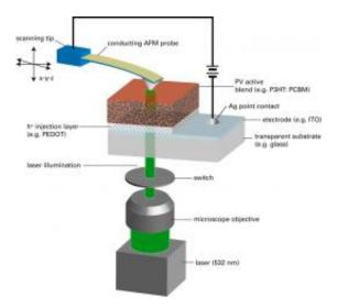
A schematic drawing of the set-up used for pc-AFM measurements.
