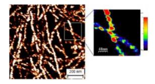
Photoconducting Atomic Force Microscopy (pc-AFM) image of a smooth polymer-nanowire based organic solar cell
