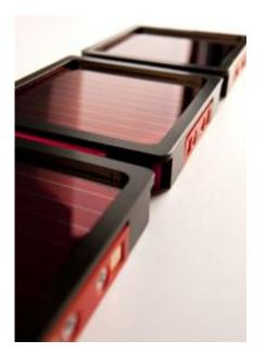
Organic solar cell modules, composed of 10 devices in monolithic series connection. The solar cells are spincoated and processed on a glass substrate. Possible applications are PV-integrated window panes.
