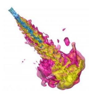
High-fidelity large eddy simulation (LES) of direct-injection processes in internal-combustion engines provides an essential component for development of high-efficiency, low-emissions vehicles. Here LES reveals how fuel from a stateof-the-art injector mixes with air inside an engine cylinder. Image credit: Joseph Oefelein and Daniel Strong, Sandia National Laboratories.
