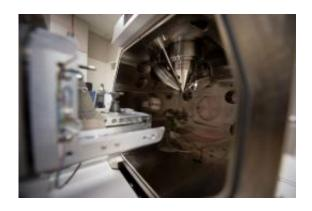
The inside of the specimen/vacuum chamber of NREL's FEI Nova 200 dual beam electron microscope used to analyze the topography of materials such as Innovalight's Silicon Ink. The instrument is used to produce site-specific sections for high spatial microstructural analysis. Credit: Dennis Schroeder
