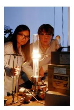
Georgia Tech graduate students Yike Hu and John Hankinson observe a high temperature furnace used to produce graphene on a silicon carbide wafer. Credit: Image Courtesy of Gary Meek
