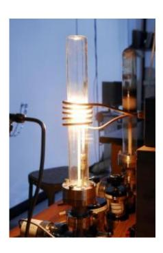
A high temperature furnace is used to produce graphene on a silicon carbide wafer. Credit: Image courtesy of Gary Meek
