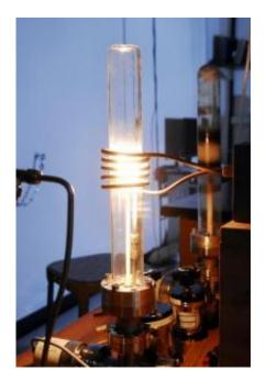
A high temperature furnace is used to produce graphene on a silicon carbide wafer. Credit: Image courtesy of Gary Meek
