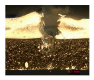
A membrane made of polyvinyl chloride-polyester (yellowish color) is punctured with a 2.5-millimeter diameter needle, and at that moment the polyurethane foam (brown) suddenly expands. Credit: Empa
