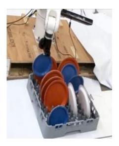
Placing dishes in a rack is a challenging task for a robot. It must identify empty spaces and place the plate in the correct upright position.
