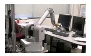
After scanning a room, a robot points to the keyboard it was asked to locate. It uses context to identify objects, such as the fact that a keyboard is usually in front of a monitor.
