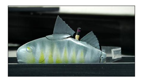
(PhysOrg.com) -- Scientists at Michigan State University are designing and studying robotic fish to be made to swim in schools in order to monitor environmental signs such as accumulations of algae and oil spills. Through the use of sensors and wireless capabilities, the fish can travel in water to collect information. But why go to all that trouble to simulate real fish if other underwater devices can be deployed for the same purpose?
