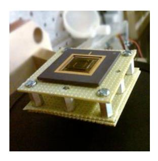
A new energy harvesting device converts low-frequency vibrations into electricity. The device, the size of a U.S. quarter, is shown mounted on a stand. Photo: Arman Hajati
