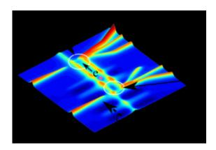
Illustration of the potential-energy landscape seen by an electron, and the potential wave produced by a sound pulse (surface acoustic wave, SAW) coming from bottom right and moving past the first dot, along the channel towards the other dot.
