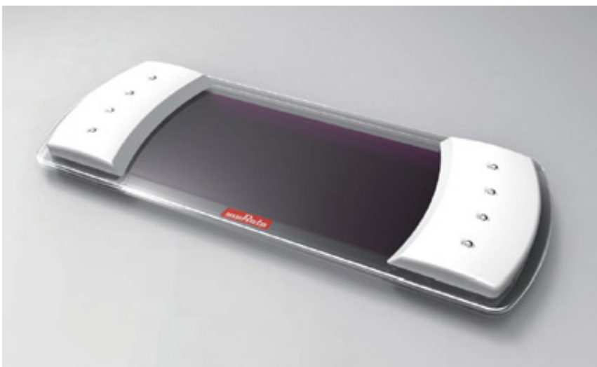
Leaf Grip Remote Controller using piezoelectric film (sample)
