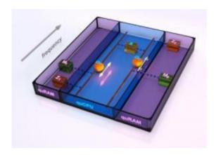
The quantum von Neumann machine: Two qubits are coupled to a quantum bus, realizing a quCPU. Each qubit is accompanied by a quantum memory as well as a zeroing register. The quantum memories together with the zeroing register realize the quRAM. Credit: Peter Allen, UCSB
