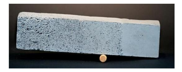
Concrete samples made by hand to illustrate the concept of density gradient in concrete. A team from the MIT Media Lab hopes to be able to print such materials with a 3-D printer.Photo: Steven Keating, Timothy Cooke and John Fernández
