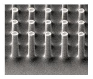
A scanning electron microscopy image of silicon nanopillars on a surfacetextured thin film for low-cost solar cells Credit: Agency for Science, Technology and Research
