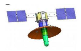
A less expensive, small-sat class system satellite with newer and more flexible technologies, TacSat-4's highly elliptical orbit augments existing geosynchronous satellites by providing near continuous communications to forward deployed forces in the high latitudes. Credit: US Naval Research Laboratory
