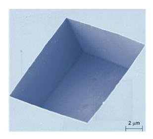
This colorized electron microscope image reveals the boxy shape of the pits the NIST team etched into the diamond surface, exhibiting their smooth vertical sidewalls and flat bottom. The pits were between 1 and 72 micrometers in size. Credit: NIST
