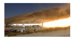
NASA and ATK's five-segment solid rocket motor fires during Development Motor-3 test in Promontory, Utah, on Sept. 8. Credit: ATK
