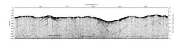
The NASA-led team used the 40-megahertz airborne sounding radar prototype to probe the desert subsurface above the Umm-El-Aish aquifer in northern Kuwait, creating this high-resolution cross section of the aquifer. The radargram shows variations in the depth of the water table from 161 to 171 feet (49 to 52 meters). Image credit: NASA/JPL-Caltech
