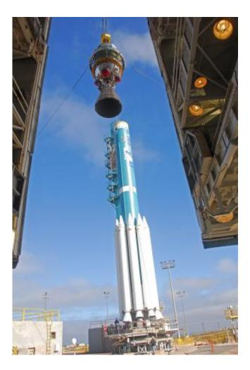
The second stage is being hoisted up onto the United Launch Alliance Delta II rocket that will launch NPP into orbit in October.Credit: NASA/Vandenberg Air Force Base
