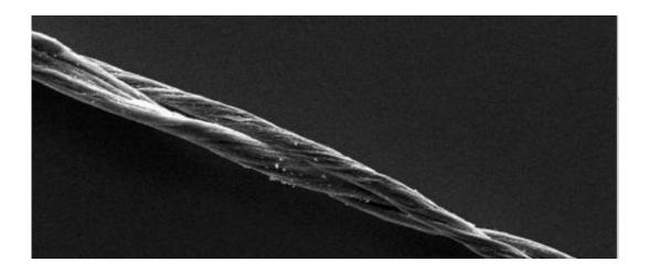
A power cable made entirely of iodine-doped double-walled carbon nanotubes is just as efficient as traditional power cables at a sixth the weight of copper and silver, according to researchers at Rice University. (Credit: Yao Zhao/Rice University)
