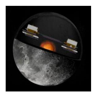
An artist's rendering of the twin GRAIL spacecraft orbiting the moon. The project uses two spacecraft flying in formation with known altitude amd separation distance to investigate the moon's gravity field in unprecedented detail. Image: NASA/JPL
