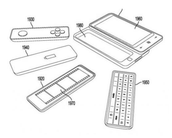
(PhysOrg.com) -- Microsoft has filed for a patent featuring slider smartphones designed to also carry interchangeable modules such as game controller, a spare battery or keyboard. The Microsoft <u>patent</u> is entitled "Mobile communication device having multiple, interchangeable
