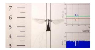
This screenshot from the video below shows the flying microrobot performing vertical flight with closed-loop control. Image credit: Néstor O. Pérez-Arancibia, et al. ©2011 IOP Publishing Ltd
