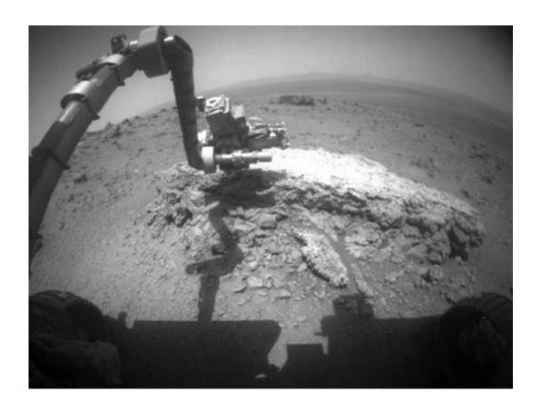
NASA's Mars Exploration Rover Opportunity used its front hazard-avoidance camera to take this picture showing the rover's arm extended toward a light-toned rock, "Tisdale 2," during the 2,695th Martian day, or sol, of the rover's work on Mars (Aug. 23, 2011). Tisdale 2 is about 12 inches (30 centimeters) tall. Image Credit: NASA/JPL-Caltech
