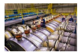
Technicians service the linear HERMES pulsed-power machine — the most powerful gamma ray producer in the world — for its next shot. Because of Sandia's nuclear responsibilities, HERMES and Saturn are kept in "warm, standby mode" for immediate testing of components. Credit: Randy Montoya
