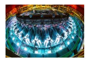
Saturn, Sandia's workhorse pulsed-power machine, delivers hard radiation during one of its milestone shots. The scarcity of jagged, lightning-like arcing between different water/metal interfaces means that the machine's water insulation is effective, and that relatively much of its electrical pulse is traveling on its intended path from the machine's circular exterior to its central target. Credit: Randy Montoya
