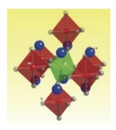
Crystal structure of complex oxide material La2MnNiO6. An ordered arrangement of Mn and Ni ions renders this material ferromagnetic with an unusual stability for operation in extreme stress environments.
