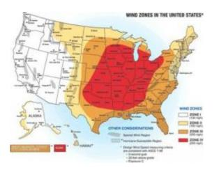
This wind zone map shows how the frequency and strength of extreme windstorms vary across the United States. Wind speeds in Zone IV (red), where the risk of extreme windstorms is greatest, can be as high as 250 miles per hour. Credit: Federal Emergency Management Agency
