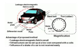
A schematic of the proposed power transfer system. This system transmits electric power thorough a capacitor composed of a steel belt and a metal plate attached to the road, and the power feed in differential mode.
