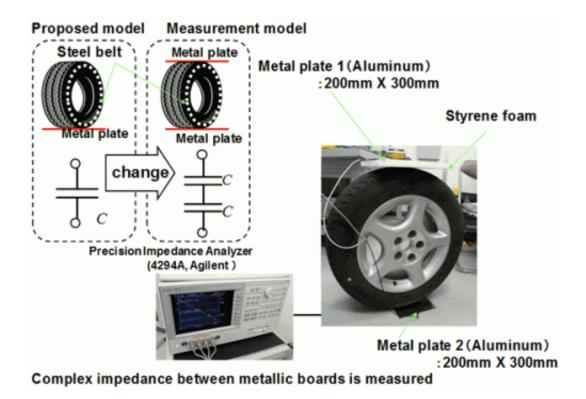
The proposed model and measurement model. As a the measurement model a metallic board were arranged above and below the tire, and the complex impedance was measured. Pieces of styrene foam of different thickness were placed between the upper surface of the tire and metallic plate. The measurement frequency was from 10 kHz to 10 MHz.
