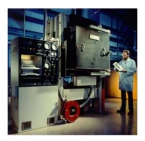
Pacific Northwest National Laboratory had just completed a materials project with Boeing and had invested in resources, including a quarter-million dollar superplastic forming press. The press allowed the team to evaluate operating conditions and aluminum alloys for superplastic forming.
