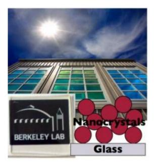
Berkeley Lab researchers have unveiled a semiconductor nanocrystal coating material capable of controlling heat from the sun while remaining transparent. This heat passes through the film without affecting its visible transmittance, which could add a critical energy-saving dimension to "smart window" coatings.
