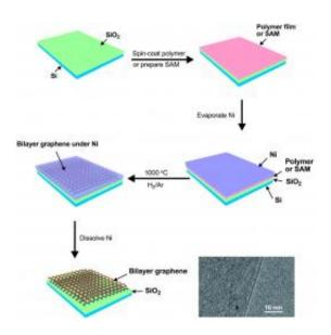
This graphic shows the process of creating bilayer graphene on an insulating substrate, skipping the need to transfer graphene from a metal catalyst. The final image, captured with an electron microscope, clearly shows two layers of graphene produced via the process. (Credit Tour Lab/Rice University)
