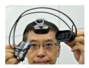
Hitachi engineer Takeshi Ogino dispays a portable 'brain-machine' interface' equipped with an optical sensor in a headset to measure prefrontal bloodstream, at the company's headquarters in Tokyo on September 14. A Japanese research team have unveiled a headset they say can measure activity in the brain and could be used to improve performance in the classroom or on the sports field.
