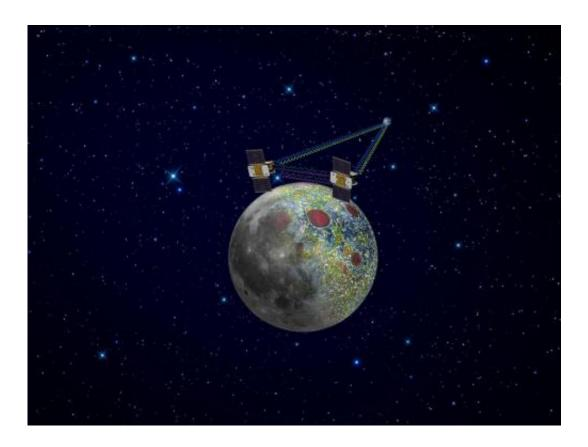
Flying in formation around the Moon, NASA's twin GRAIL spacecraft will make precise measurements of the lunar gravitational field. Credit: NASA/JPL-Caltech
